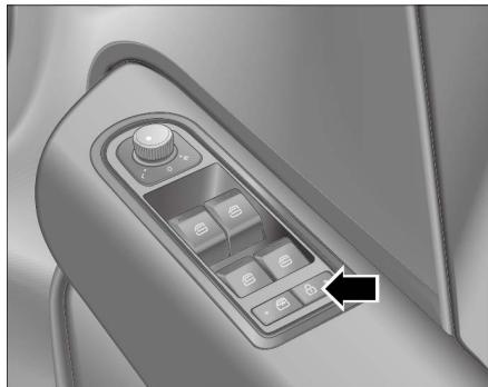
The central locking button is located on the driver door window regulator switch panel for convenient operation.
