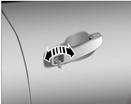
4. Insert the mechanical key, rotate the door lock cylinder counterclockwise to unlock and clockwise to lock.
