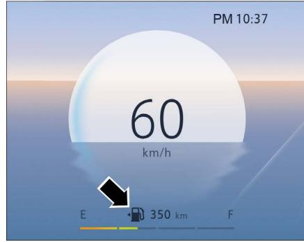
The fuel gauge is located at the lower part of the speedometer. The fuel gauge is equally divided into 4 sections. When the keyless start/stop button is in the "RUN" mode, the fuel gauge displays the amount of fuel remaining in the fuel tank. The indication of "E" to "F" implies that the fuel tank varies from empty to full. When the keyless start/stop button is in the "OFF" mode, the current remaining amount of fuel cannot be displayed.
