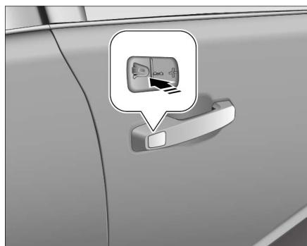
3. Pull up the driver door handle and use your fingers to push the protective cover in the direction of the arrow on the inside of the door handle. Remove it to
