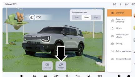
By clicking the centre console display sidebar or clicking the vehicle settings icon > Common on the centre console display. The ON/OFF of the HDC function can be set.
