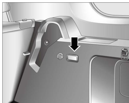
The trunk lamp automatically switches on when the tailgate is opened, and automatically switches off when the tailgate is closed.
