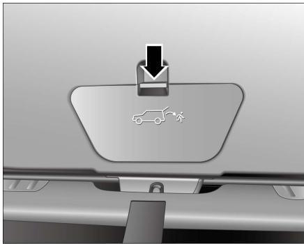
1. Fold the rear seats into the trunk and push down to remove the tailgate latch cover in the middle at the bottom of the tailgate.
