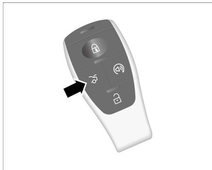
The tailgate is in the closed state. Briefly press the tailgate button on the smart key twice to automatically open the tailgate.
