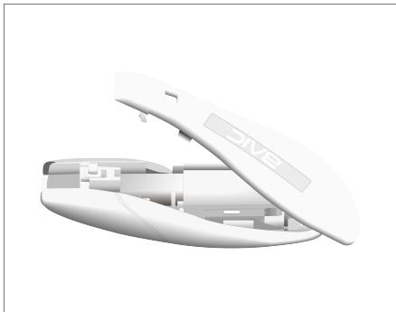
2. Use a suitable tool to pry open the back cover of the smart key.
