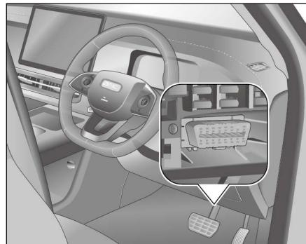
The diagnostic interface is located under the IEC.
