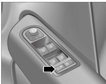
When the button is pressed down, the passenger side electric window regulator switch will not be able to control the window. It is activated when the window lock switch is pressed again.
