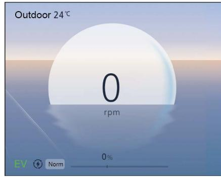
Displays the drive motor power and the energy recovery power.
