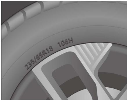
Check the vehicle tyre information, and get correct tyre specifications and dimensions.
