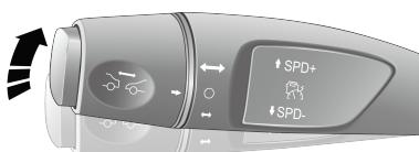
After activating ACC, toggle the cruise control lever upward, and the cruise speed will increase in increments of 5 km/h. When you toggle the cruise control lever upward for the first time, the ACC system will adjust
