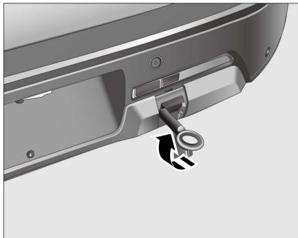
3. Screw the towing eye clockwise into the threaded hole and use a hard metal rod or similar tool to secure it tightly.
