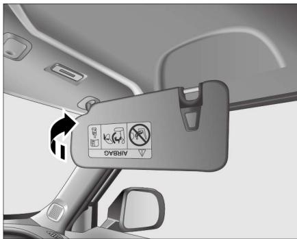
First flip the sun visor downward, then detach its hinge from the clasp before rotating it toward the window to block sunlight coming through the door side.
