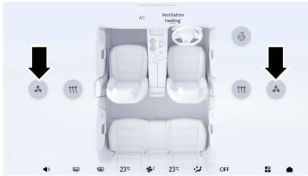
Slide up at the bottom edge of the main interface of the centre console display to enter the air conditioning control interface > ventilation heating, or tap the air conditioning control button > ventilation heating in the Dock bar at the bottom of the centre console display. Tap the seat ventilation button to activate the seat ventilation function. Repeat the button to switch between the following gears: gear 3, gear 2, gear 1, and off.
