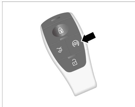
When ATS is activated and within a distance of less than 15m (open space), briefly press the search button on the smart key, and the vehicle will emit a search sound and light prompt.
