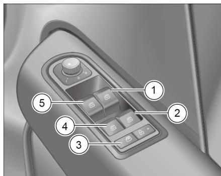
The power window switch is located on the driver door window regulator switch panel.
