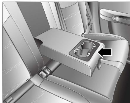
Pull down the centre armrest of the seat to open the centre armrest of the rear seat. When folding up the centre armrest, push it into the backrest of the rear seat.
