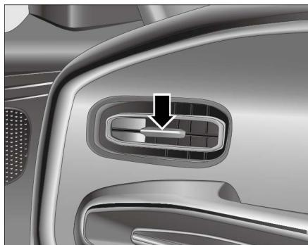
Left vent: Slide right to open the vent and slide left to close it.
