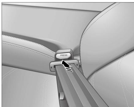
Slowly pull the seat belt out of the retractor, then insert the latch plate into the buckle until you hear a ‘click’ sound, then pull back on the seat belt to make sure that it locks reliably.
