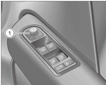
The exterior rearview mirror adjustment switch ① is located at the front end of the driver's side power window switch.
