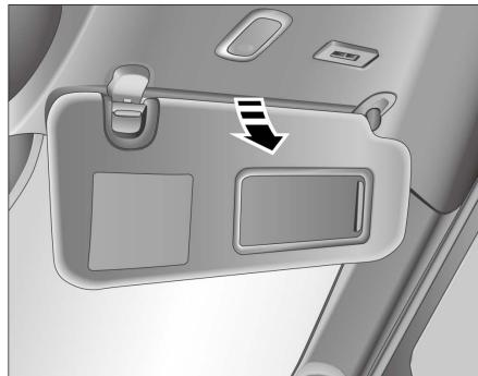
Both the driver-side and front passenger-side sun visors can be flipped downward from their respective brackets to block sunlight entering through the windshield.
