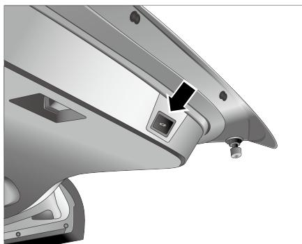
When the tailgate is in the open state, press the close switch on the tailgate to automatically close it.
