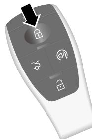
To lock all doors, briefly press the lock button on the smart key with all doors, bonnet and tailgate properly closed.
