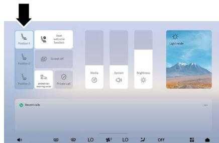
After completing the seat position adjustment, swipe downward from the top edge of the centre console display main interface to enter the minus one screen. Tap any of the three positions in the seat memory area to save the current seat position.
