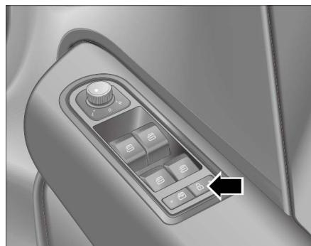
The central locking button is located on the driver door's window regulator switch panel for convenient operation.
