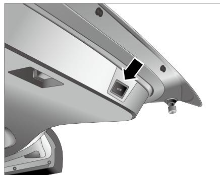
Open the tailgate, adjust it to the desired position, and then press and hold the tailgate inner switch for 3 seconds. A prompt sound will sound once to indicate the completion of the tailgate opening height setting (50%~100%).
