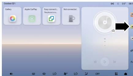
Tap the AVM icon on the sidebar of the centre console display to go to the AVM interface. Tap the OFF button in the upper right corner to turn off the AVM system.
