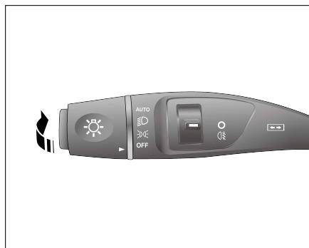
When the low beams go on, push the light control lever forward to illuminate the high beams and pull the light control lever back again to turn off the high beams.
