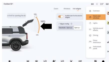
By tapping the vehicle settings icon > Doors and windows > Power tailgate on the centre console display. The tailgate opening height can be set.
