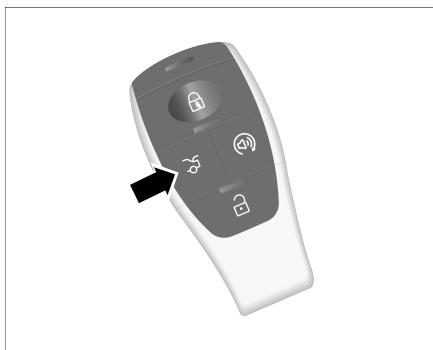
The tailgate is in the open state. Briefly press the tailgate button on the smart key twice to automatically close the tailgate.
